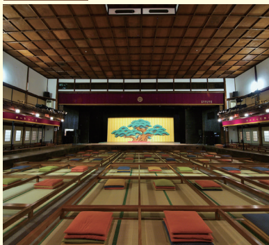
Naraku The revolving stage of 16m in diameter and elevator are manually operated
